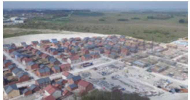
As of week ending 12 April 2019, over 200 timber frames stand on the Larkhill site, with more than 180 roofed and in excess of 155 brick wrapped.
